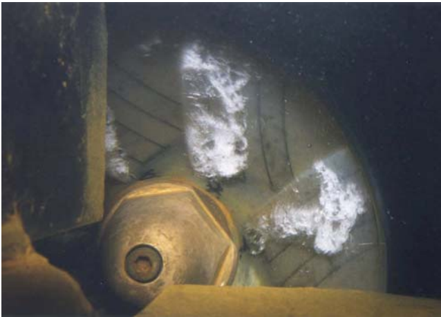
Figure 1.5 Cavitation at the impeller inlet
