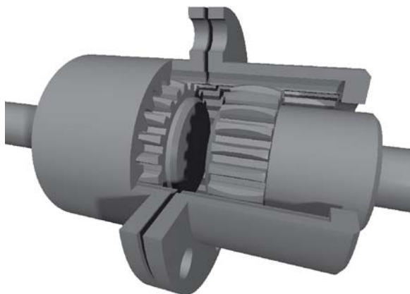
Figure 5.4 Typical gear coupling
